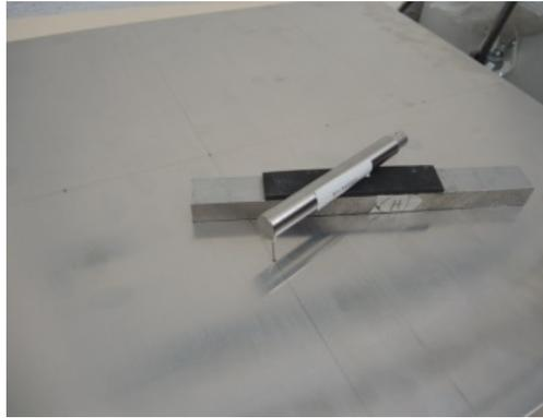
Figure 10 - Photograph of the pinhole microprobe used for the determination of the upper wall wind-tunnel wall-pressure fluctuations under a TBL excitation.
