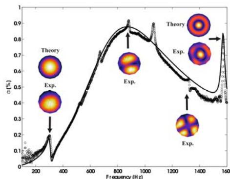
Figure 1- Sound absorption coefficient of the MPPA predicted assuming an elastic (solid black) MPP and measured using the two-microphone method (black circles).
