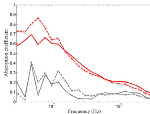
Figure 12 - Third-octave averaged absorption curves for a number of partitions undergoing a TBL excitation: plain front panel (solid grey: calculated; dashed grey: measured), micro-perforated front panel (solid red: calculated; dashed red: measured).
