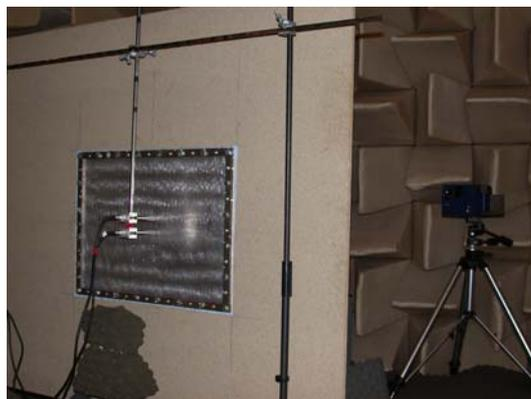
Figure 7 - Experimental set-up for determination of the absorption and transmission properties of the insulating MPP partition, with the laser vibrometer situated in front of the backing side.
